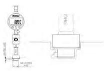
Measurement of dovetail seat face width
